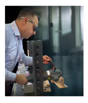
Blast Tehnik laser cleaning machine makes rust, coatings and impurities evaporate in seconds. I could not believe what I was seeing when I first tried this machine. An ergonomic design, lightweight laser gun and quick-setup menu makes it user friendly. At the same time it is ultimately precise and removes only desired coated areas without any damage on base material, which is especially important for our pharmacy process equipment.
